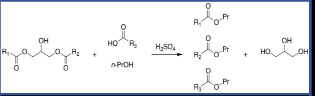
Fig. 3: Fischer esterification of free fatty acids and trans esterified triglyceride with 1-propanol and sulfuric acid to produce glycerol and three esters.
