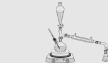
Fig. 3 - Steam distillation set up
