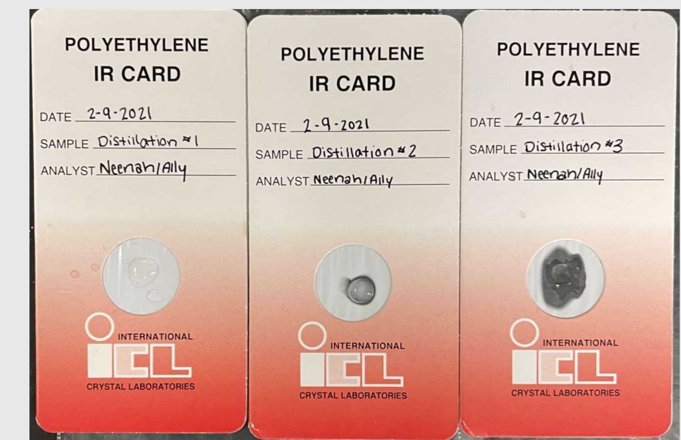
Figure 3 displays the three polyethylene FTIR cards that contained samples of the three batches of distillate. These cards were then placed into the FTIR machine to examine the wavenumber and absorbance of distillates/
